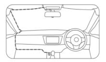
Please use a pry tool to conceal the power line under the roof upholstery and seal the rubber ring along the A-pillar.
