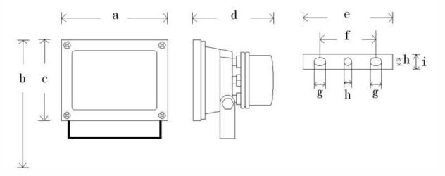
a: 228mm, b: 185mm, c: 128mm, d: 205mm, e: 90mm, f: 13mm, g: 35mm, h: 10mm, j: 30mm
