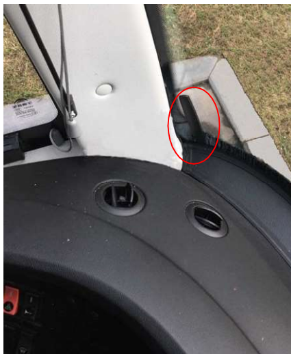
Figure 2-24 Inside installation of Mobile Network Antenna
