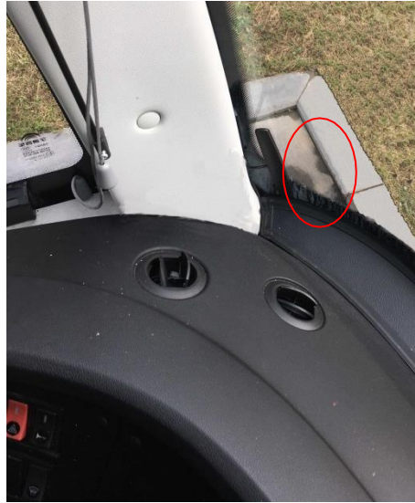
Figure 2-17 Inside installation of Mobile Network Antenna
