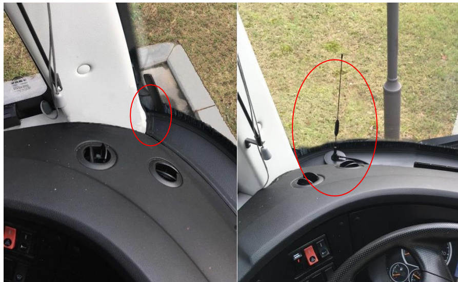
Inside installation of Mobile Network Antenna
